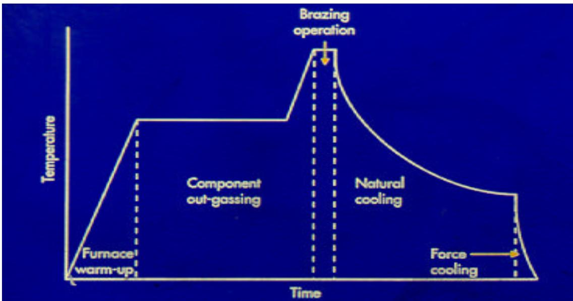
Figure 1.15 The “One Shot Seal Off Cycle
