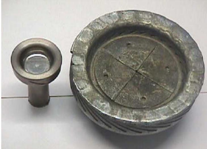
*Figure 1.12 Comparison of size of contact for 12kV 20kA rating.*
