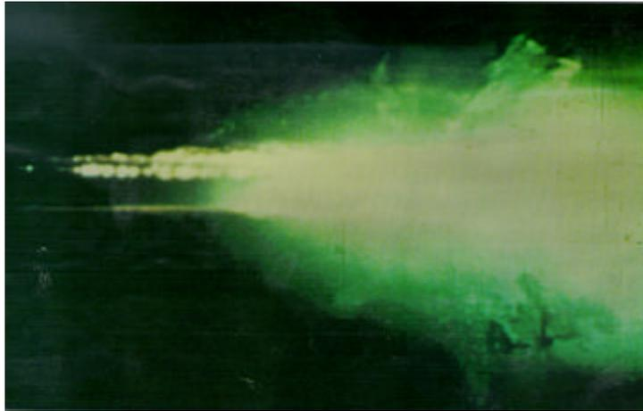
*Figure 1.8 Still from HS film @ 10,000pps showing constricted arc on plain contact geometry (55mm diameter disc) CLR carrying @5000A. The liquid spilling over the edge of the contact is boiling chromium and copper.*
