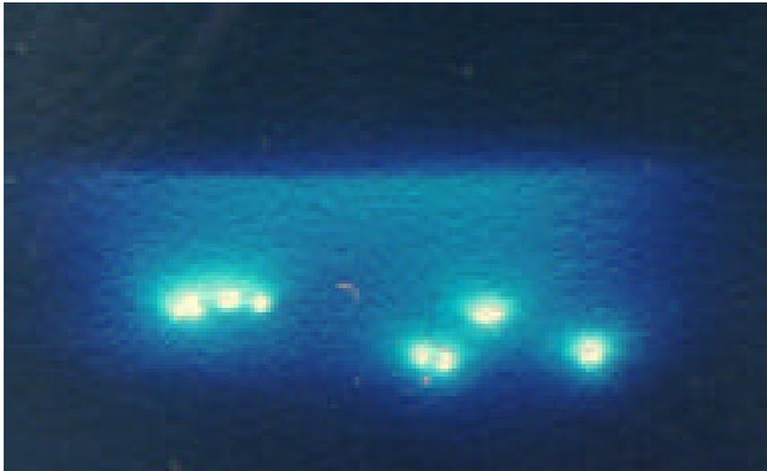
*Figure 1.7. Still from High Speed film @ 10,000pps showing cathode spots on plain contact geometry (55mm diameter disc) CLR carrying @200A*
