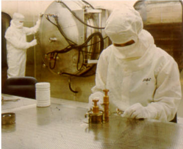
*Figure 1.17 This shows One Shot Seal Off of V204 vacuum interrupters in a clean room in South Africa. After assembly the interrupters are loaded into a vacuum furnace and brazed and sealed at the same time.*
