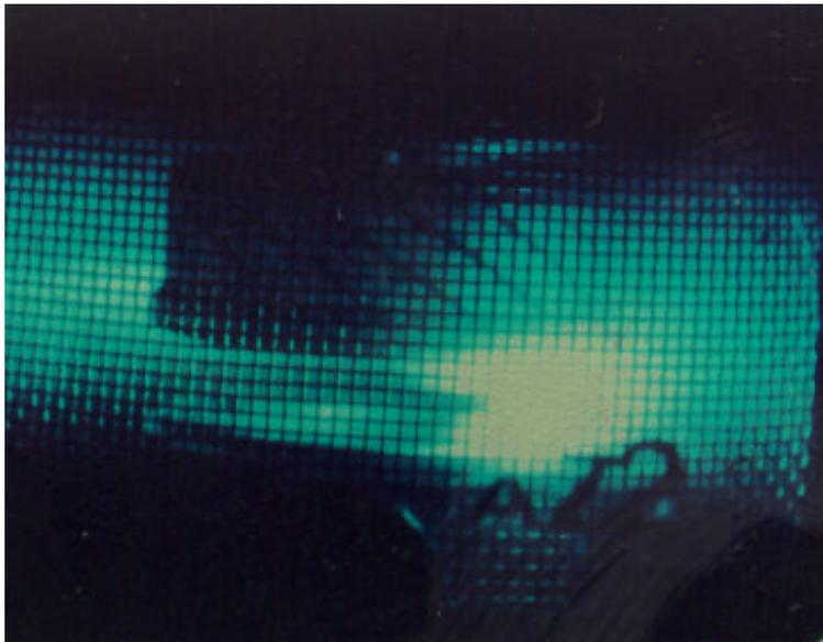
*Figure 1.11. Still photo from a High Speed film @ 5,000 pps showing a 55mm diameter RMF contact interrupting 31.5kArms @12kVrms.*
