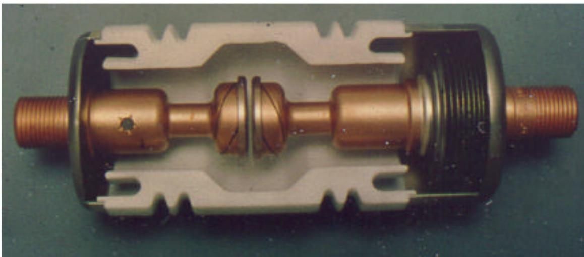
*Figure 1.14. The V204 interrupter which was the world's first "shieldless" vacuum interrupter. It is rated at 12kV;20kA.*
