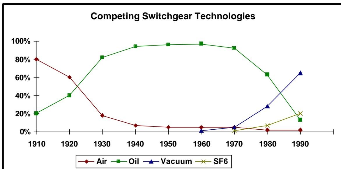
Figure 1.2 The competing switchgear technologies in Medium Voltage Switchgear during the 20th Century.
