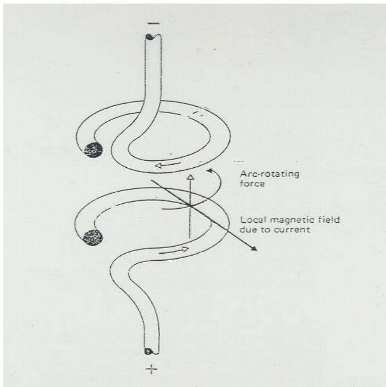
*Figure 1.9. The principle of operation of a Radial Field Contact.*
