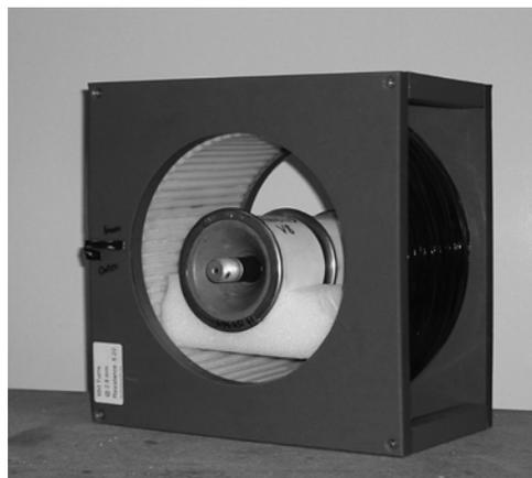
**Fig. 5. A vacuum interrupter in the solenoid coil.**
