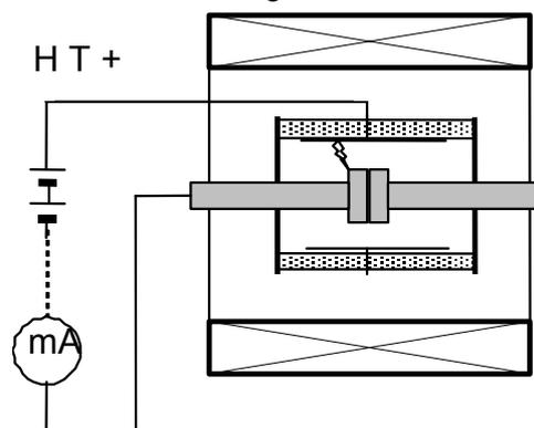
**Fig. 6. A schematic Magnetron Circuit.**
