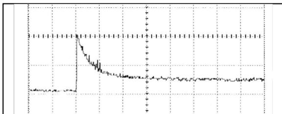
Figure 7. Typical magnetron pulse from an interrupter.
