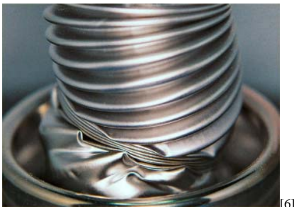
Fig. 5. A bellows damaged during assembly into the circuit breaker
