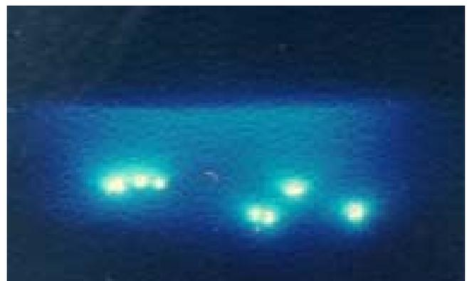
Figure 2. Natural Diffuse Mode. High speed film @ 10,000 pps on plain butt contact 200A@12kV.
