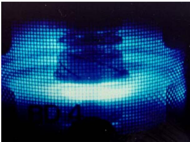
Figure 6 “Folded Petal” RMF Contact interrupting 20kA @12kV.
