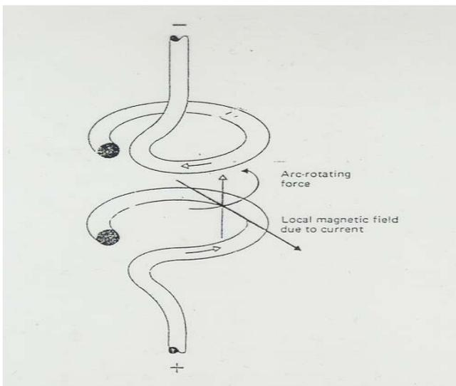
Figure 4. Principle of operation of Radial Magnetic Field device.
