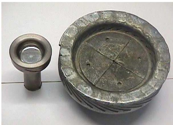
Figure 7 “Comparison of sizes of Contrate and Folded Petal contact for the same rating (20kA@12kV).
