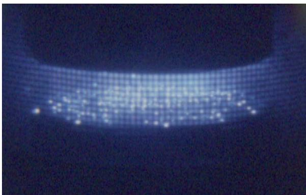
Figure 8. Diffuse arc using AMF contact interrupting 31.5kA@12kV
