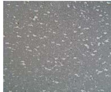
Figure 12 Photomicrograph of Tungsten-carbide Silver
