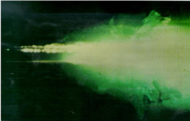
Figure 3. Plain butt contact carrying 5kA@12kV Boiling Copper and Chromium can be clearly seen.
