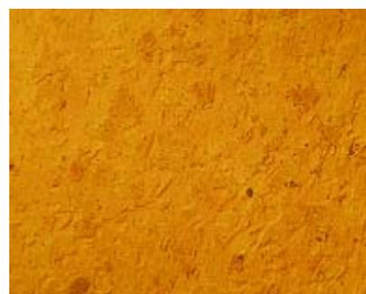
Figure 10. Photomicrograph of Copper Bismuth.
