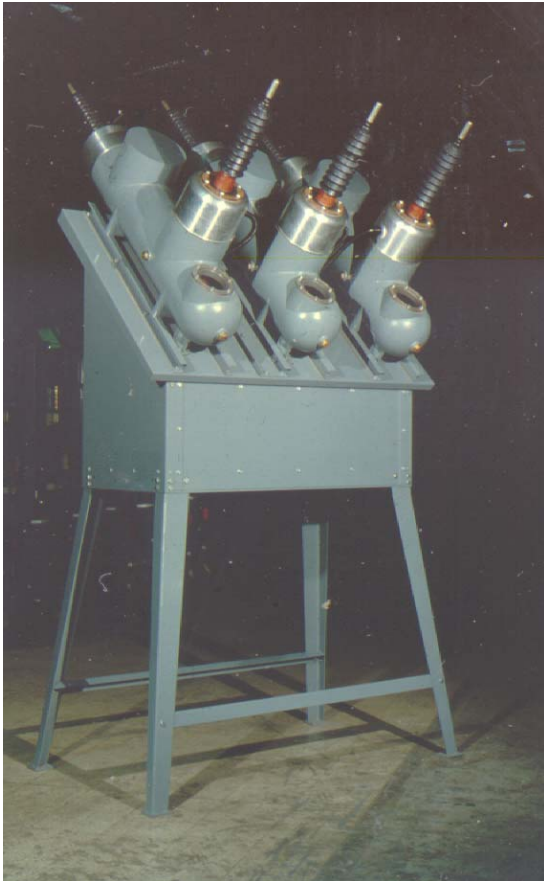
Figure 3. OX circuit breaker c.1982. The three tanks each containing a vacuum interrupter insulated in SF 6 gas can clearly be seen. The windows in the tanks which acted as pressure relief in case of internal arc are at the bottom of each tank. The mechanism is housed inside the box underneath the circuit breaker. Inside each tank is one V8 type vacuum interrupter rated at 38kV; 25kA; 1250A.
