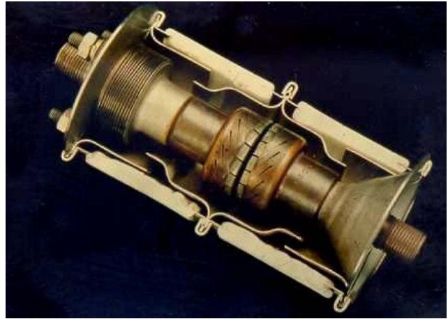
Figure 6. V803 12kV:25kA:1250A vacuum interrupter designed in the late 1970's showing welded construction of bellows and insulator flanges
