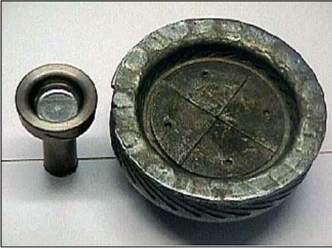
Fig. 9. Comparison of size of contacts for 12 kV at 20 kA rating from 1968 to 1984.
