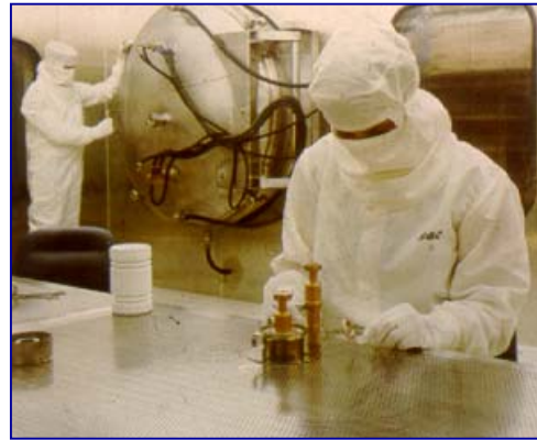
Fig. 13. This shows "One Shot Seal Off" of V204 vacuum interrupters in a clean room in South Africa. After assembly the interrupters are loaded into a vacuum furnace and brazed and sealed at the same time.
