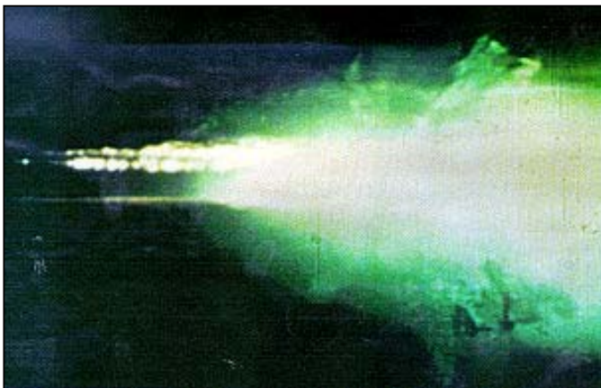
Fig.6. Still frame from High Speed Film at 10,000 fps showing constricted arc on plain contact geometry CLR carrying 5000 A. The liquid spilling over the edge of the contact is boiling chromium and copper. (VIL circa 1970)
