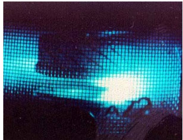
Fig.8. Still photo from a High Speed film at 5,000 fps showing a 55 mm diameter RMF contact interrupting 31.5kArms (VIL circa 1982)
